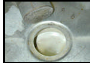
Water level is correct when it is above the drain neck.
