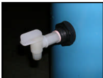
Valve in open position.
