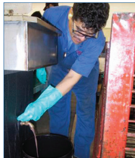
Figure 3. A worker is shown purging oil from the collection chamber in the Grease Gator.
