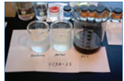
Figure 2. The "before and after" cleaning solutions appear to be similar from the Grease Gator.
