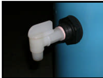
Valve in closed position.
