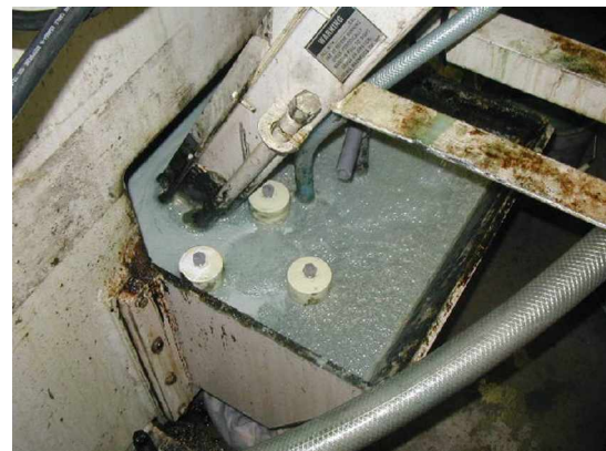
Broach Coolant Sump after 2 hours of Grease Gator Purification
