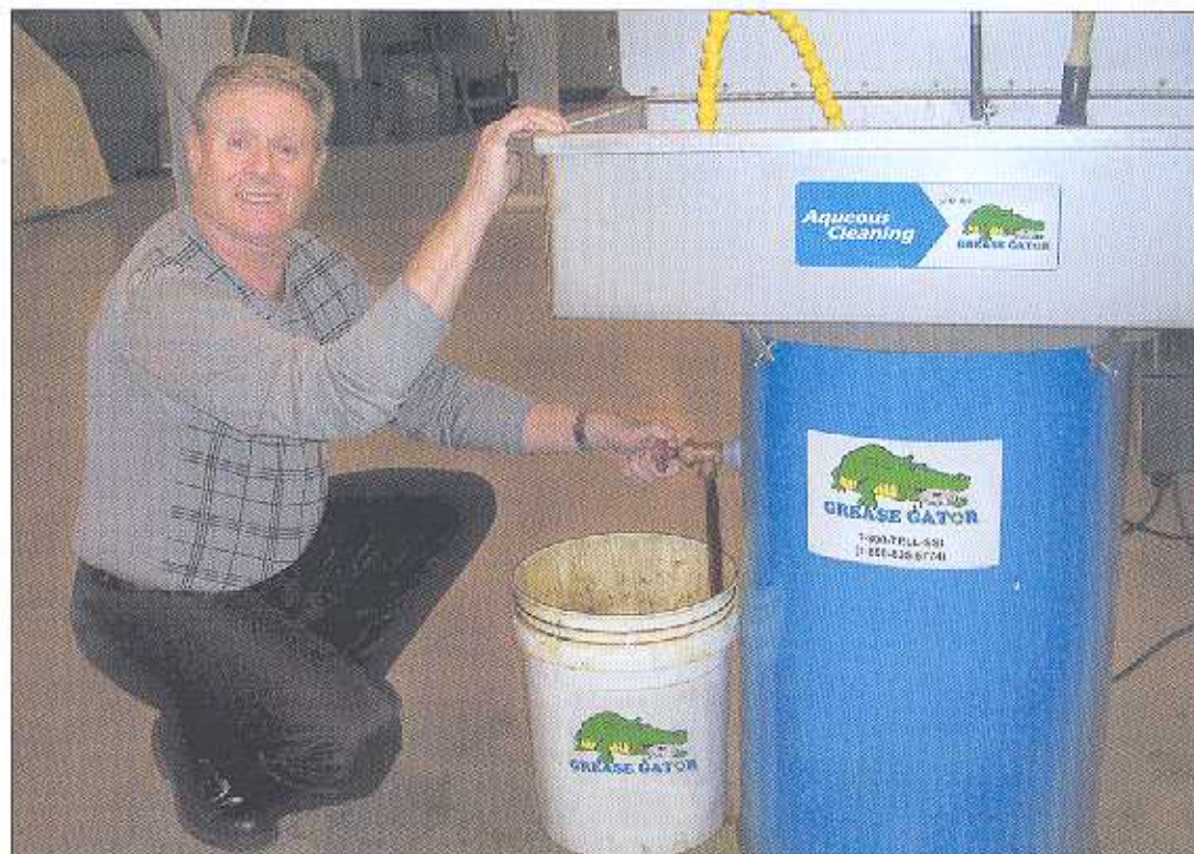
Steve Rundell, president of Solvent Systems International, shows how a spigot on the side of the Grease Gator releases oil that has been separated from other ingredients after the Gator is used to clean dirty machine parts. The company buys the waste oil back from its customers.
